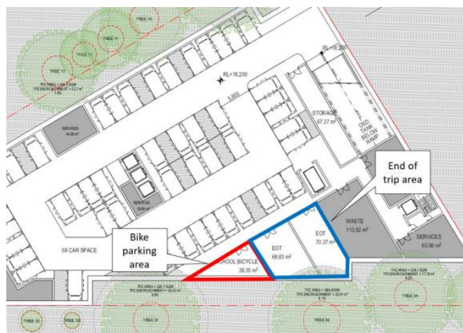
Figure 41 Bicycle parking and end of trip facilities
